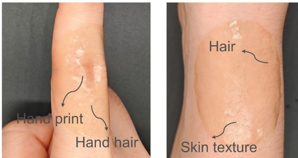
**Fig. S14.** CPA hydrogel was highly transparent and soft-and-thin, it could be even seen the hair, hand prints, and skin texture underneath the sample.
