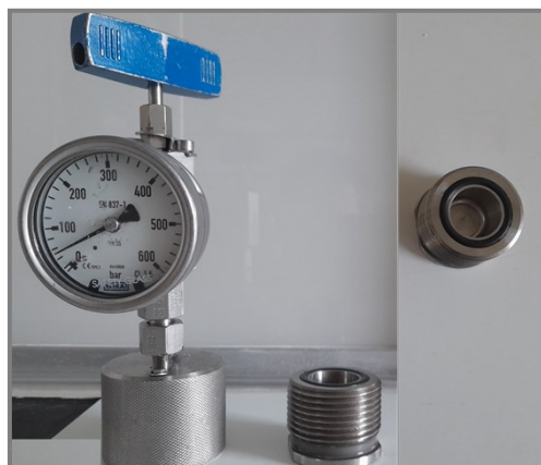
Figure S22. stainless-steel autoclave with a nominal volume of 12 ml.
