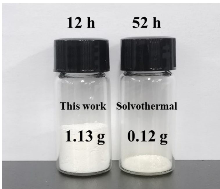
Figure S32. Yields of \text{Ti}_6\text{tbbz}_{10} clusters synthesized with autoclaves of the same size by solid-phase (left) and solvothermal method (right) .
