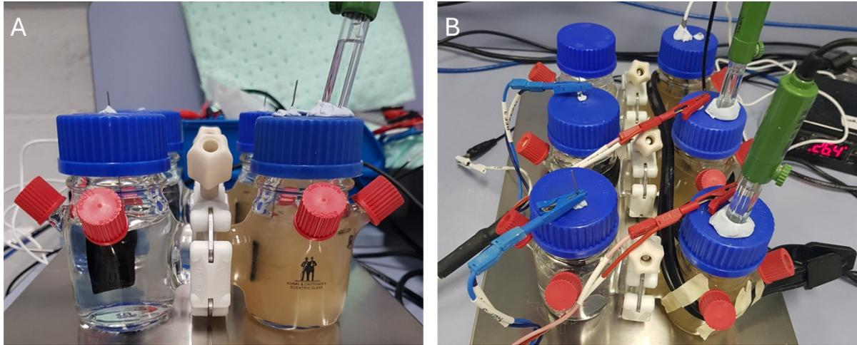
Suppl Fig 4 Construction of anodic electrofermentation systems employed. A. Side view of system setup with M9Y media in the working chamber. B. Top down view of anodic electrofermentation systems with electrodes connected to Biologic potentiostat via crocodile clips.
