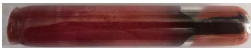
Fig.S2 Photograph of the quartz tube filled with WP after heating to 800°C, holding for 10 hours, and then slowly cooling to room temperature.
