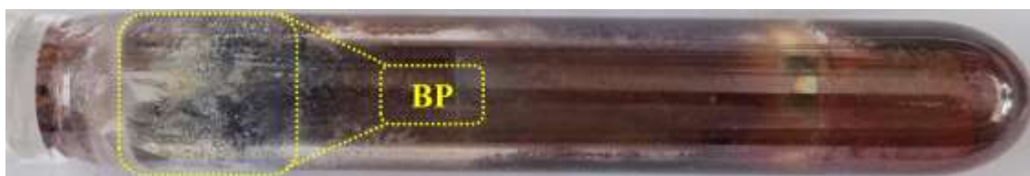
Fig.S8 Physical images of BP prepared by quenching the reaction with liquid nitrogen.
