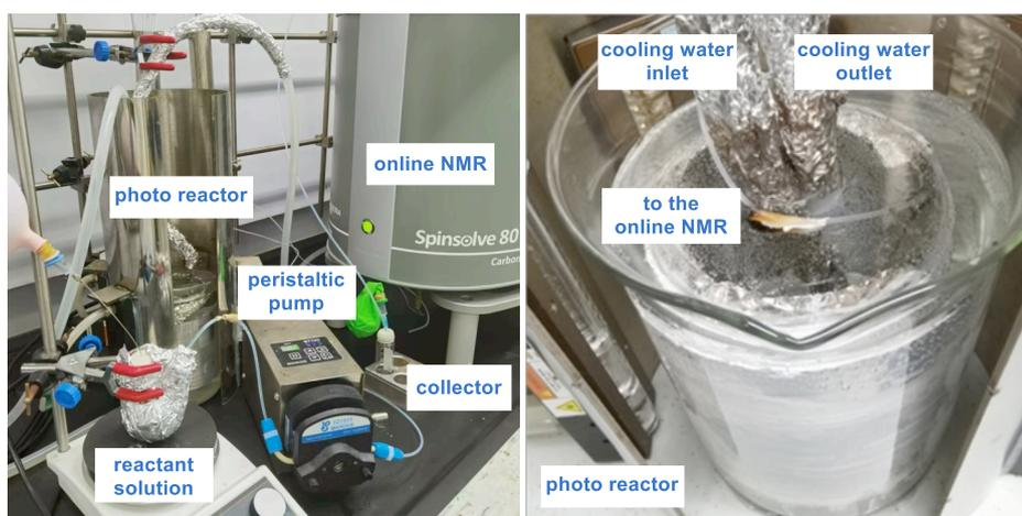
Figure S1. The continuous-flow reaction set-up.
