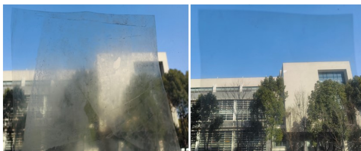
Fig. S5 After glutenin phase transition incubation, photo of PET plastic partially washed with high-pressure water gun (left) and photo of PET plastic sheet washed clean with high-pressure water gun (right).
