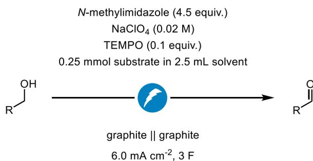
Scheme S1. Standard conditions for TEMPO-mediated alcohol oxidations in an ElectraSyn 2.0 electrolysis set-up.
