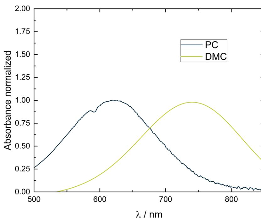
Figure S1: Normalized UV-vis spectra of Betaine 30 in propylene carbonate (PC) and dimethyl carbonate (DMC).
