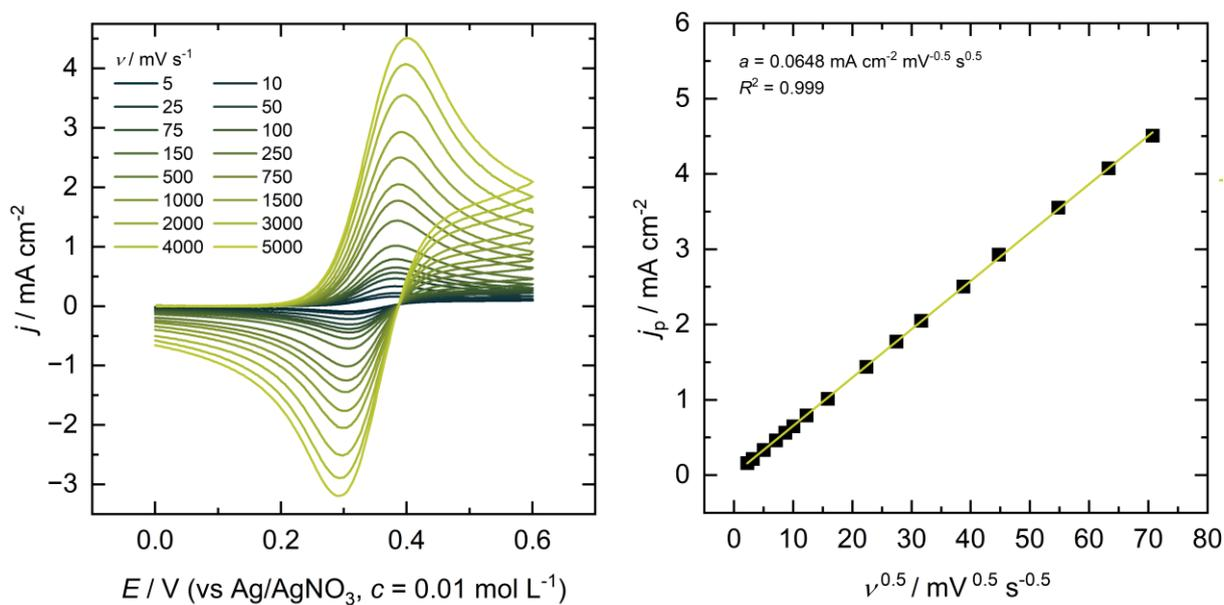
Figure S7: Cyclic voltammetry of 2.5 mM TEMPO in an electrolyte consisting of 0.1 M Bu<sub>4</sub>NBF<sub>4</sub> in PC-DMC (3:7, w/w).
