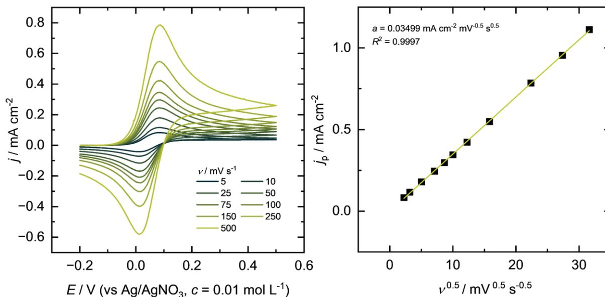
Figure S20: Cyclic voltammety of 2.5 mM Ferrocene in an electrolyte consisting of 0.1 M Bu<sub>4</sub>NBF<sub>4</sub> in PC.
