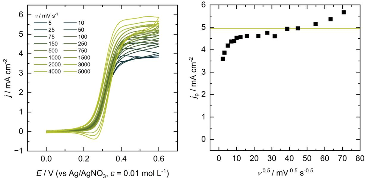
Figure S17: Cyclic voltammetry of 2.5 mM TEMPO with 100 mM 4-MBA and 450 mM 1-NMI in an electrolyte consisting of 0.1 M Bu<sub>4</sub>NBF<sub>4</sub> in PC-DMC (6:4).
