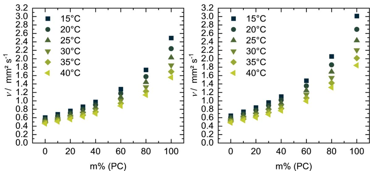
Figure S2: Kinematic viscosity of PC-DMC mixtures at different temperatures without (left) and with 0.1 M  $\text{Bu}_4\text{NBF}_4$  (right).
