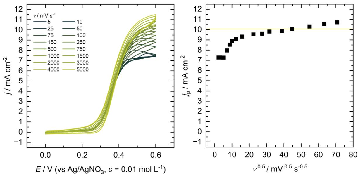
Figure S14: Cyclic voltammetry of 2.5 mM TEMPO with 100 mM 4-MBA and 450 mM 1-NMI in an electrolyte consisting of 0.1 M  $\text{Bu}_4\text{NBF}_4$  in PC-DMC (2:8).
