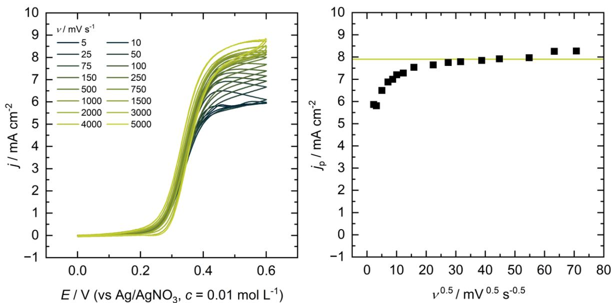
Figure S16: Cyclic voltammetry of 2.5 mM TEMPO with 100 mM 4-MBA and 450 mM 1-NMI in an electrolyte consisting of 0.1 M  $\text{Bu}_4\text{NBF}_4$  in PC-DMC (4:6).
