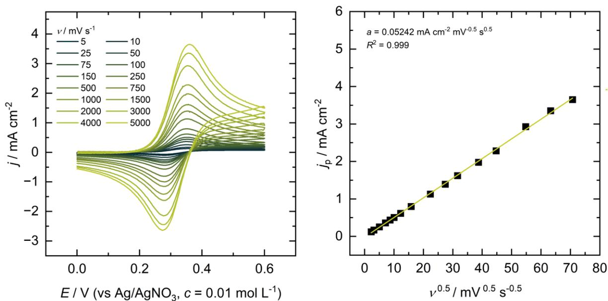
Figure S9: Cyclic voltammetry of 2.5 mM TEMPO in an electrolyte consisting of 0.1 M Bu<sub>4</sub>NBF<sub>4</sub> in PC-DMC (6:4, w/w).
