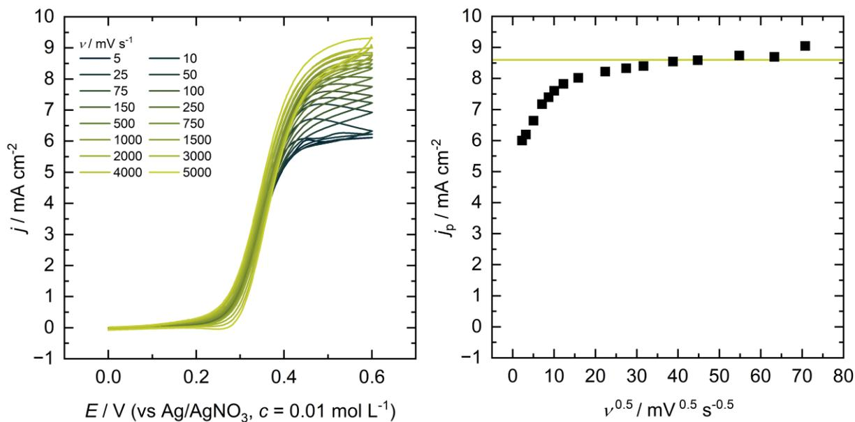
Figure S15: Cyclic voltammetry of 2.5 mM TEMPO with 100 mM 4-MBA and 450 mM 1-NMI in an electrolyte consisting of 0.1 M  $\text{Bu}_4\text{NBF}_4$  in PC-DMC (3:7).
