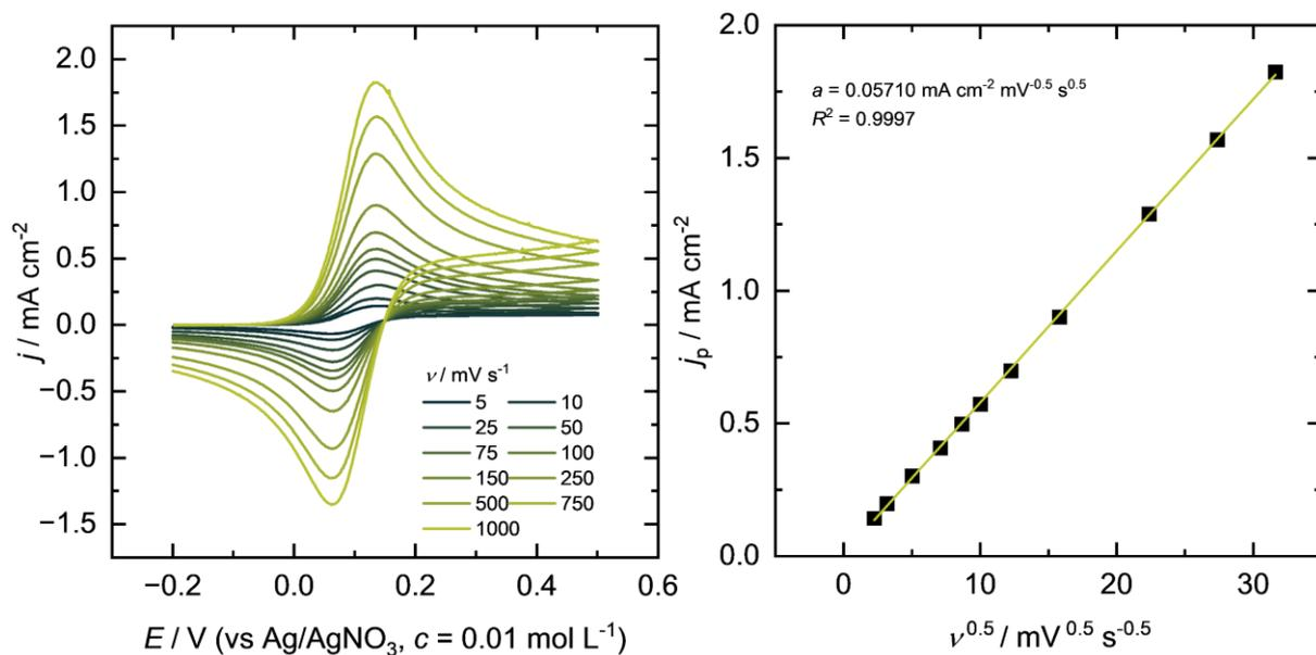
Figure S23: Cyclic voltammetry of 2.5 mM Ferrocene in an electrolyte consisting of 0.1 M Bu<sub>4</sub>NBF<sub>4</sub> in PC-DMC (4:6).
