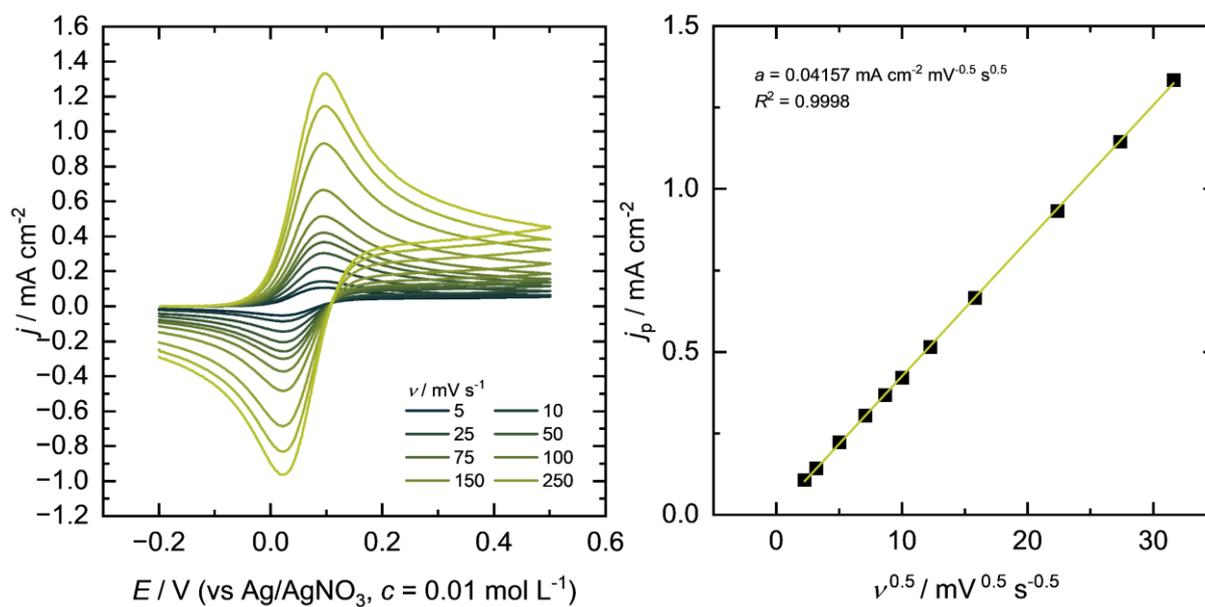
Figure S21: Cyclic voltammety of 2.5 mM Ferrocene in an electrolyte consisting of 0.1 M Bu<sub>4</sub>NBF<sub>4</sub> in PC-DMC (8:2).
