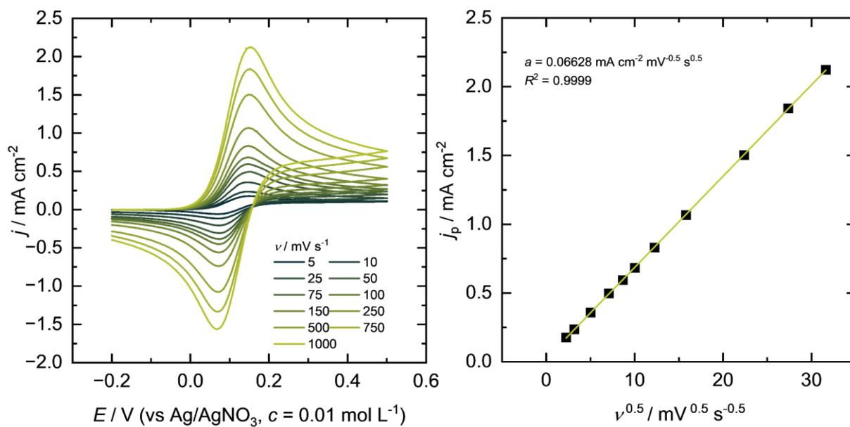
Figure S24: Cyclic voltammetry of 2.5 mM Ferrocene in an electrolyte consisting of 0.1 M Bu<sub>4</sub>NBF<sub>4</sub> in PC-DMC (3:7).
