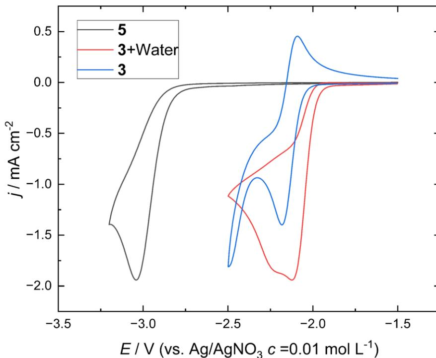
Figure S27: CVs of DPMC (**5**), benzophenone, and benzophenone in the presence of water in PC-DMC (2:8);  $c(\text{Bu}_4\text{NBF}_4) = 0.1 \text{ M}$ ,  $c(\text{analyte}) = 5 \text{ mM}$ ,  $c(\text{H}_2\text{O}) = 0.56 \text{ M}$ .
