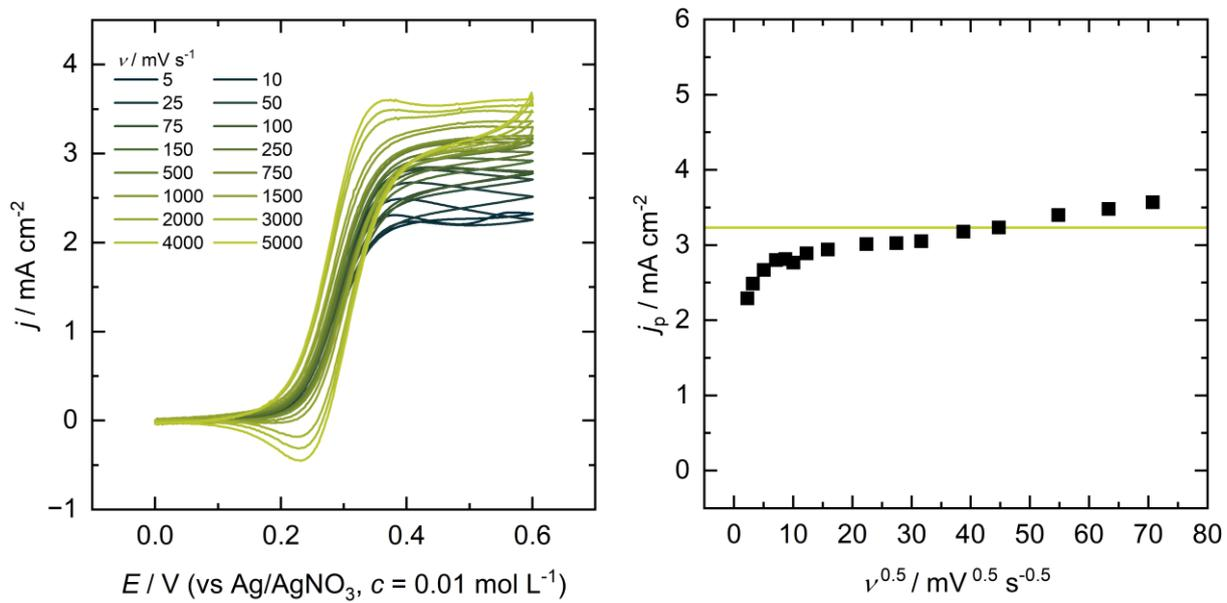
Figure S19: Cyclic voltammetry of 2.5 mM TEMPO with 100 mM 4-MBA and 450 mM 1-NMI in an electrolyte consisting of 0.1 M  $\text{Bu}_4\text{NBF}_4$  in PC-DMC (10:0).
