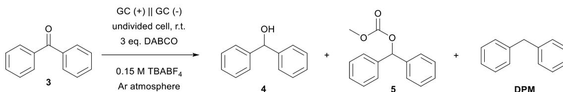
Table S7. Results of cathodic reduction of benzophenone in different solvents using an undivided cell. Working electrode: GC, counter electrode: GC,  $n(\text{substrate}) = 0.5$  mmol,  $c(\text{Bu}_4\text{NBF}_4) = 0.12$  M,  $n(\text{DABCO}) = 1.5$  mmol (3 equiv.).
