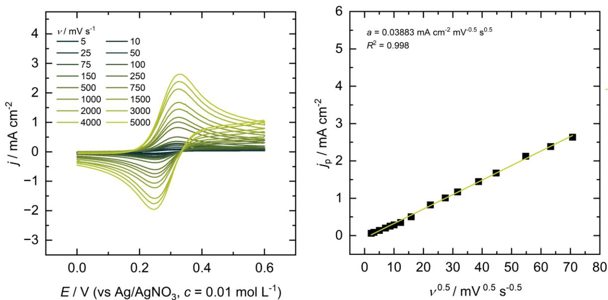
Figure S11: Cyclic voltammetry of 2.5 mM TEMPO in an electrolyte consisting of 0.1 M Bu<sub>4</sub>NBF<sub>4</sub> in PC.
