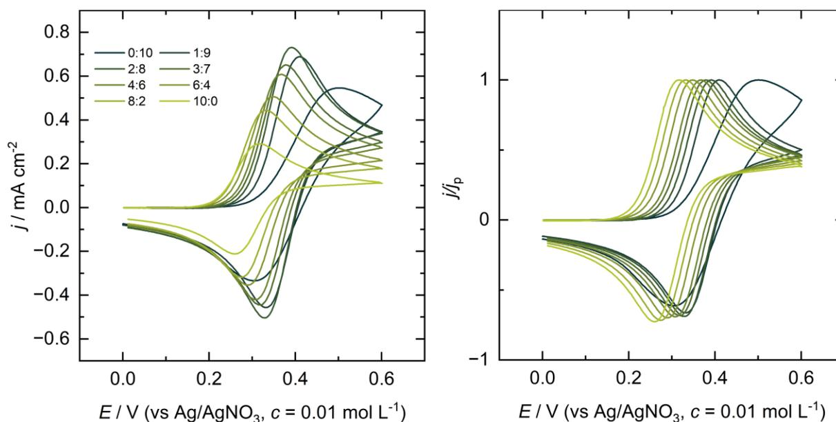
Figure S12. Comparison between the CVs of 2.5 mM TEMPO recorded in different mixtures of PC-DMC at 100 mV s<sup>-1</sup> (supporting electrolyte: 0.1 M Bu<sub>4</sub>NBF<sub>4</sub>).
