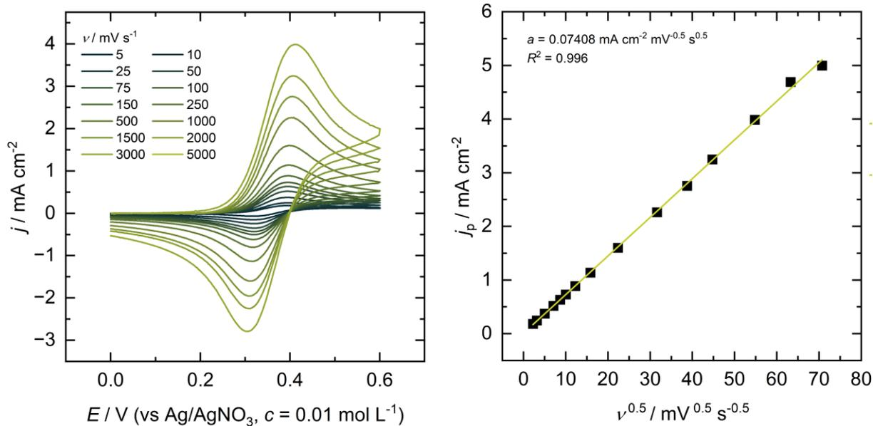
Figure S6: Cyclic voltammetry of 2.5 mM TEMPO in an electrolyte consisting of 0.1 M Bu<sub>4</sub>NBF<sub>4</sub> in PC-DMC (2:8, w/w).
