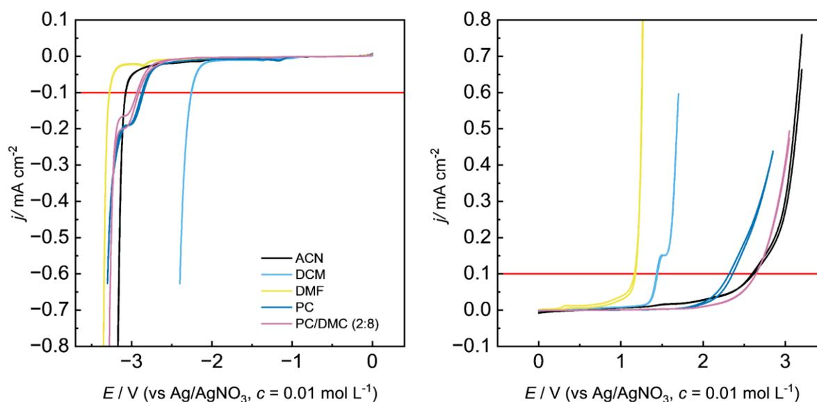
Figure S3: Blank CVs using different solvents in combination with 0.1 M Bu<sub>4</sub>NBF<sub>4</sub> as a supporting electrolyte for determining the electrochemical window at  $v = 10 \text{ mV s}^{-1}$ .
