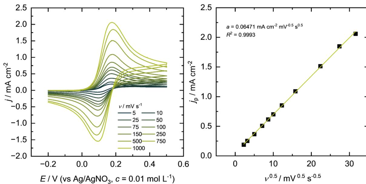
Figure S26: Cyclic voltammetry of 2.5 mM Ferrocene in an electrolyte consisting of 0.1 M Bu<sub>4</sub>NBF<sub>4</sub> in PC-DMC (1:9).
