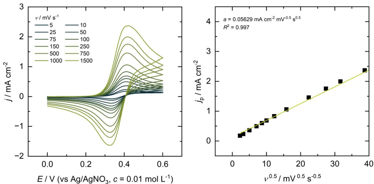
Figure S5: Cyclic voltammetry of 2.5 mM TEMPO in an electrolyte consisting of 0.1 M  $\text{Bu}_4\text{NBF}_4$  in PC-DMC (9:1, w/w).
