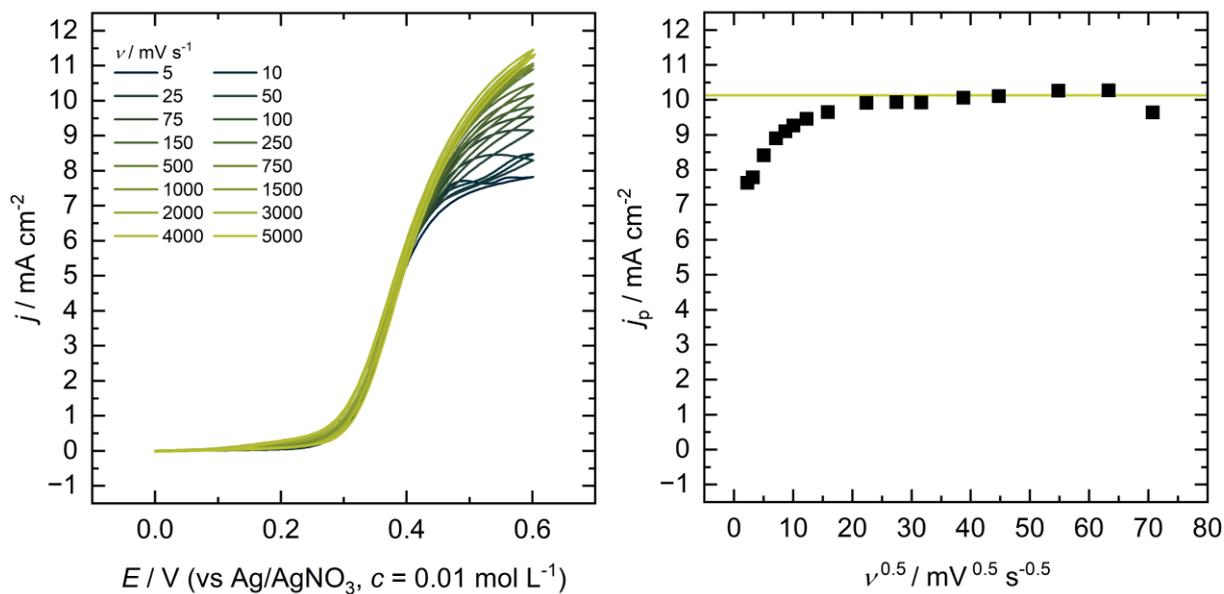
Figure S13: Cyclic voltammetry of 2.5 mM TEMPO with 100 mM 4-MBA and 450 mM 1-NMI in an electrolyte consisting of 0.1 M  $\text{Bu}_4\text{NBF}_4$  in PC-DMC (1:9).
