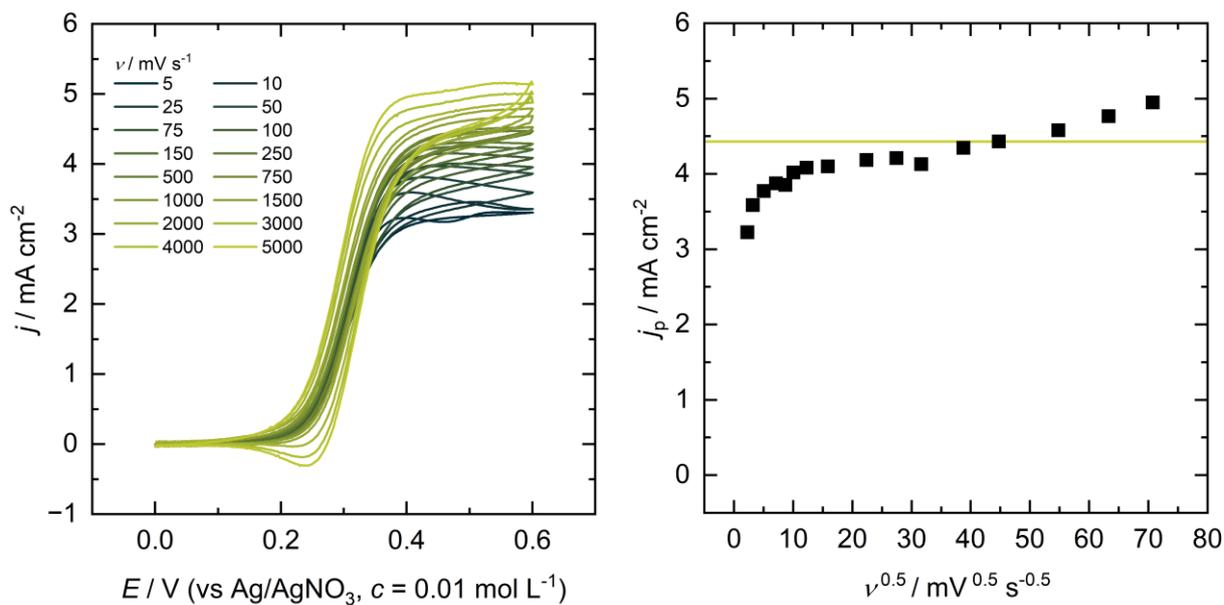
Figure S18: Cyclic voltammetry of 2.5 mM TEMPO with 100 mM 4-MBA and 450 mM 1-NMI in an electrolyte consisting of 0.1 M Bu<sub>4</sub>NBF<sub>4</sub> in PC-DMC (8:2).
