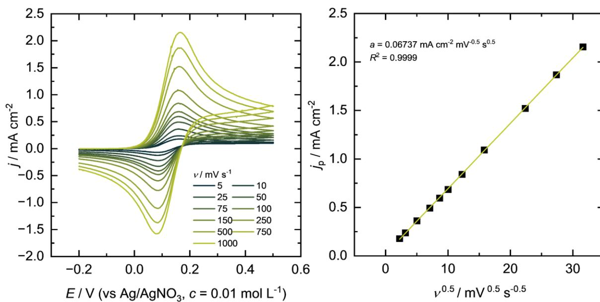
Figure S25: Cyclic voltammetry of 2.5 mM Ferrocene in an electrolyte consisting of 0.1 M Bu<sub>4</sub>NBF<sub>4</sub> in PC-DMC (2:8).
