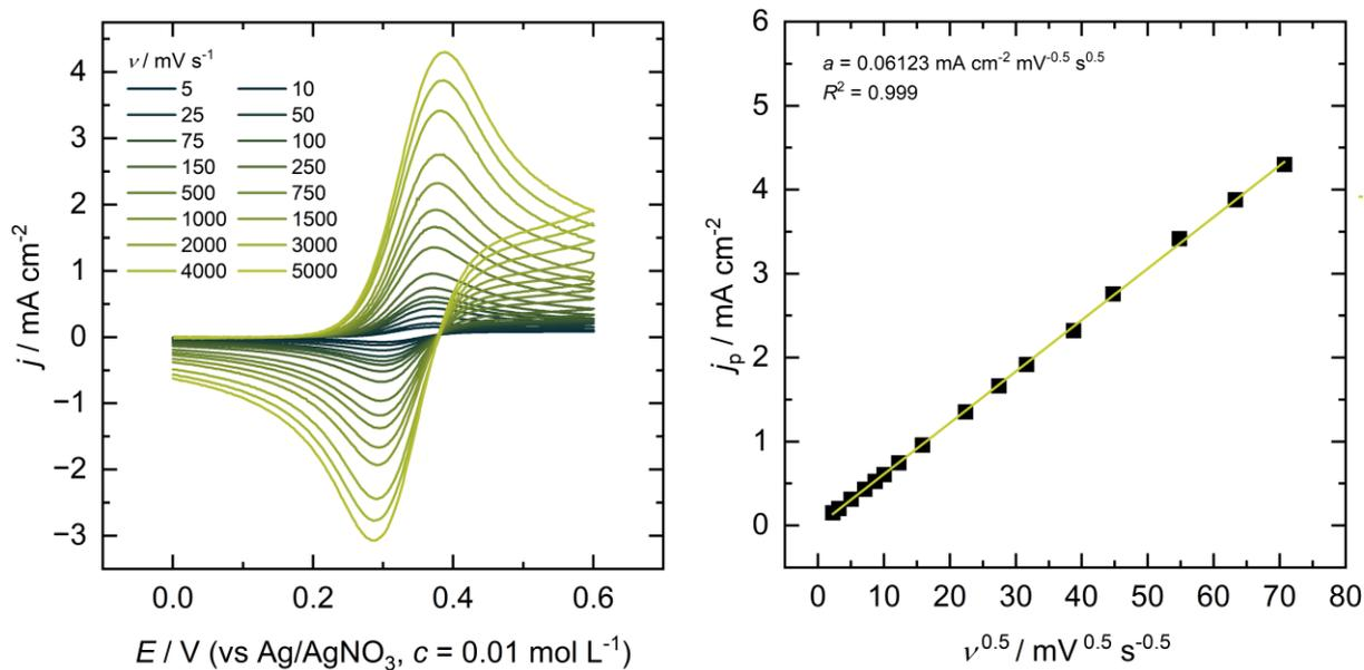
Figure S8: Cyclic voltammetry of 2.5 mM TEMPO in an electrolyte consisting of 0.1 M Bu<sub>4</sub>NBF<sub>4</sub> in PC-DMC (4:6, w/w)
