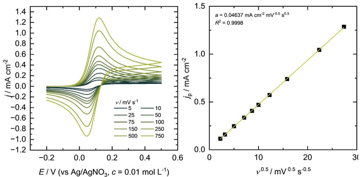
Figure S22: Cyclic voltammetry of 2.5 mM Ferrocene in an electrolyte consisting of 0.1 M Bu<sub>4</sub>NBF<sub>4</sub> in PC-DMC (6:4).
