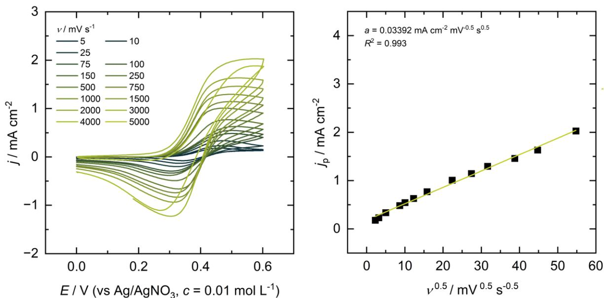
Figure S4. Cyclic voltammetry of 2.5 mM TEMPO in an electrolyte consisting of 0.1 M  $\text{Bu}_4\text{NBF}_4$  in DMC.
