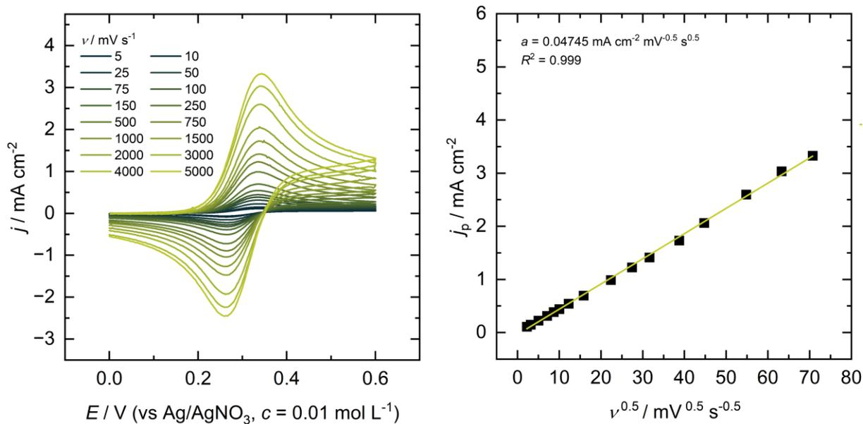
Figure S10: Cyclic voltammetry of 2.5 mM TEMPO in an electrolyte consisting of 0.1 M Bu<sub>4</sub>NBF<sub>4</sub> in PC-DMC (8:2, w/w).
