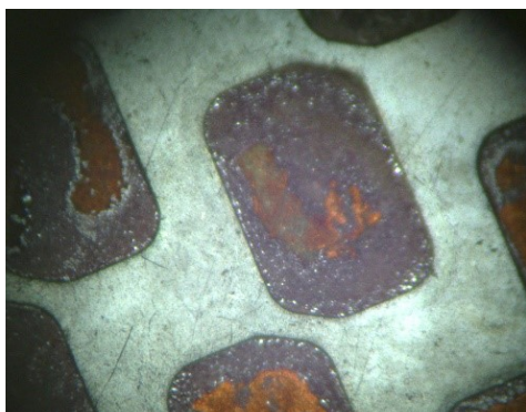
Figure S8 Optical microscope photo of CPU board after hydrothermal reaction without O 2 in the reaction system.
