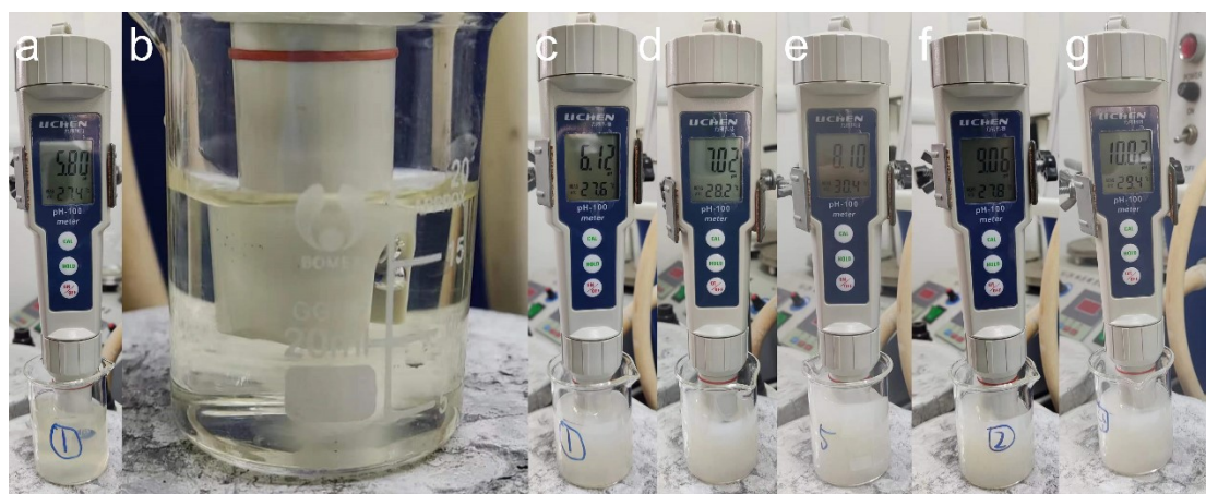
Fig. S19 Pictures of different pH in the synthesis of ZIF-93: (a) Initial pH, (b) pH=5, (c) pH=6, (d) pH=7, (e) pH=8, (f) pH=9, and (g) pH=10.
