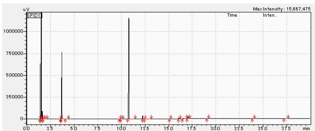
Figure S13. GC chromatograms of resultant mixtures for depolymerization of PET sheets through transesterification with ethanol using 3 mol % of FeBr 3 at 180 °C for (top) 18 h and (bottom) 30 h.
