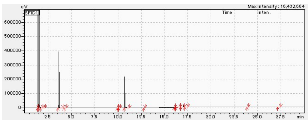
Figure S9. GC chromatograms of resultant mixtures for depolymerization of PET yellow textiles (65 % PET and 35 % cotton) through transesterification with ethanol using 5 mol% of \text{FeCl}_3 at 180 °C for (top) 12 h and (bottom) 16 h.
