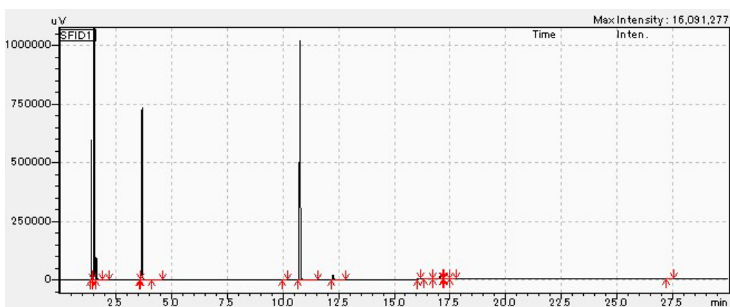
Figure S5. GC chromatograms of resultant mixtures for depolymerization of PET sheets through transesterification with ethanol using 5 mol % of \text{FeCl}_3 at 160 °C for (top) 18 h, (middle) 18 h, and (bottom) 24 h.
