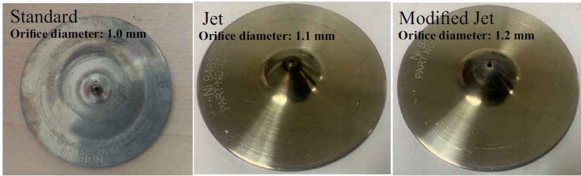
Figure S1 Exterior comparison of the Standard cone, Jet cone and modified Jet cones
