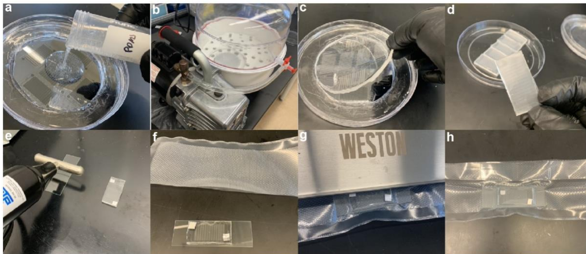
Figure S1. The fabrication and storage of microfluidic chips. (a) The PDMS elastomer and curing agent are mixed at a ratio of 10:1 and poured onto the master mold. (b) The PDMS is degassed using a vacuum pump. (c) After incubation, the PDMS slab is cut and removed. (d) Individual chips are excised and isolated. (e) Chips are bound to standard microscope slides via oxygen plasma treatment. (f) Vacuum-sealable bags are prepared for vacuum sealing. (g) The chips are vacuum sealed. (h) The chips are stored in vacuum-sealable bags until use.
