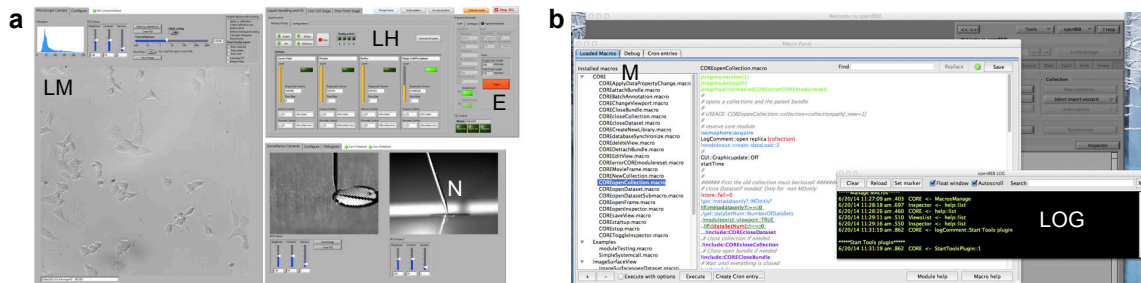
Fig. SI-4 Screenshots of the graphical user interface (GUI) of the control software (a) and the macro and logging system of openBEB 1 (b). a) GUI of the control software used for single-cell lysis. The microscopy view (LM) is shown with HEK cells, the panel for the liquid handling (LH), and the observation camera with the nozzle (N). b) The instrument can be automatized by an extensive, domain-specific macro language by openBEB's macro subsystem; here, the integrated macro editor (M) is shown, additionally providing an extensive logging facility (LOG).
