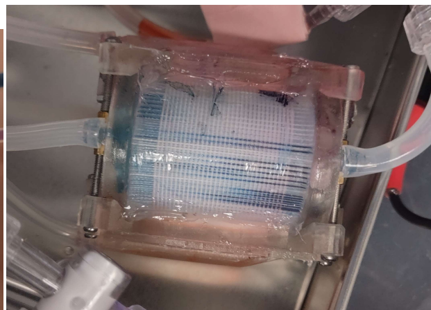
Figure S4A (left): Device A during leak testing. There is a leak between the blood phase and gas phase in one half of the device, resulting in blue dye entering the blood phase. That half of the device was blocked off.
