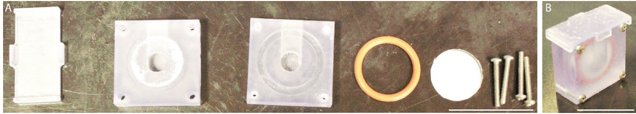
Figure S4. Photographs of A) the components and B) the assembled holder were used to evaluate the membrane permeability of the HUVEC cells deposited in the SGS scaffolds. A) Each component was printed on a Form Labs 3B+ 3D printer. The components from left to right include the lid, to maintain sterility, side 1 of the reservoirs, side 2 of the reservoirs, a 25 mm (inner diameter) silicone O-ring (McMaser-Carr), to prevent leakage, the scaffold that gets placed between the two reservoirs, either cell-free or cell-containing, and the 20 mm 4-40 316ss screws used to hold the device together (McMaster-Carr). The screw holes in side 2 of the reservoir were threaded with a 4 - 40 tap (McMaster). B) The assembled holder, which places the cell containing membrane perpendicular to the benchtop. The scale bars in both photographs represent 40 mm.
