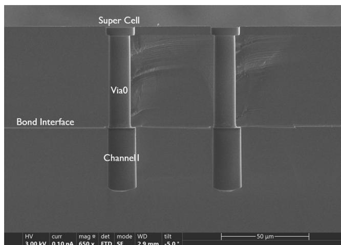
Figure S3: (a) Scanning electron microscopy (SEM) image of Channel2/Via1/Channel1 cross section; (b) Wafer-level sound acoustic microscopy (SAM) image after bonding of the first two Si wafers; (c) Scanning electron microscopy (SEM) image of Channel1/Via0/Supercell cross section.
