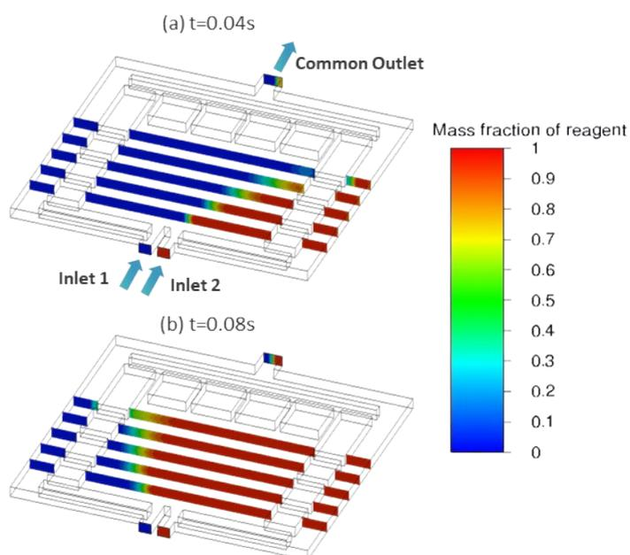
Figure S5: the cross-sectional views of reagent mass fraction in 5 planes at  $-50$ ,  $-25$ ,  $0$ ,  $25$ , and  $50 \mu\text{m}$  offset from the center of the cavity at  $t = 0.04$  and  $0.08$  s. The numerical simulation details were the same as described in Figure 4.
