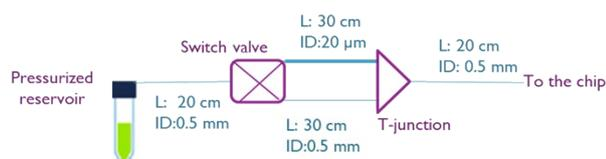
Figure S4: (a) schematic of the experimental set-up to test the fast switching of the proposed supercell design. Images are captured with
