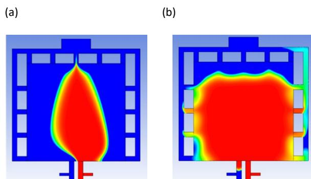
Figure S1: Comparison between (a) a non-optimized supercell with a outlet busbar where all the outlet channels have the same resistance and (b) an optimized design of a supercell where the widths of the outlet channels to the main cavity are adapted to modulate their resistances.
