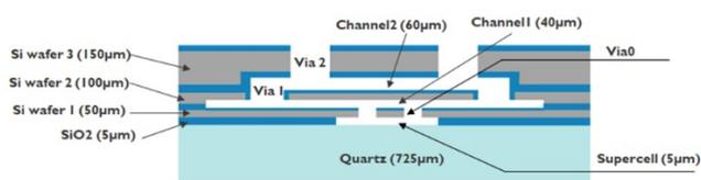
Figure S2: Schematic cross section (not to scale) of the fabricated fluidic device with the heights of the individual layers indicated.
