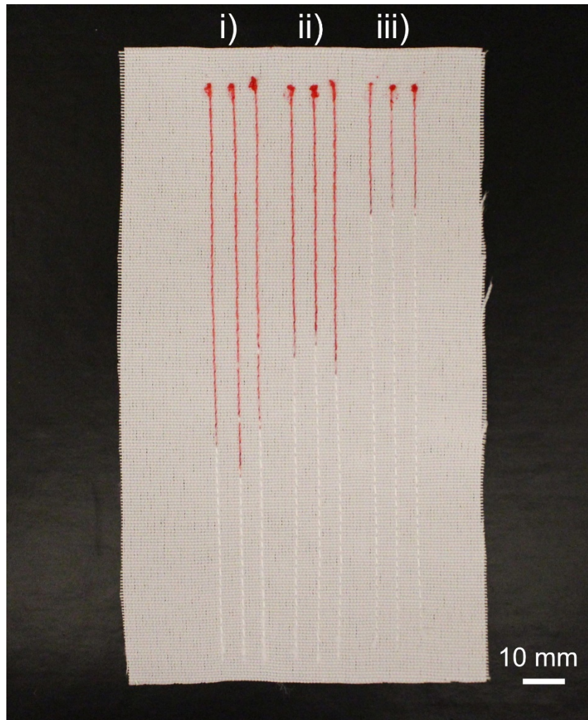
Figure S1: Comparison of flow distance in stitched microfluidic channels in the woven fabric using straight stitches with i) Coolmax® as both spool and bobbin thread, ii) Coolmax® as spool thread and non-wicking nylon thread as bobbin thread, and iii) nylon thread as spool thread and Coolmax® as bobbin thread (the latter stitched with the fabric upside down so that the microfluidic channels are visible in all three cases from the same side).
