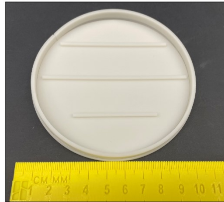
Fig. S1 (a) The design of pneumatic chamber mold by Solidworks. The chamber height and width are 2 mm and 2mm, respectively; (b) 3-D printed mold for creating PDMS replica.
