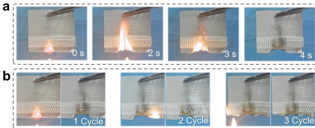
**Fig. S5** (a) The FEP adhered to the surface of the substrate extinguishes the flame. (b) The FEP extinguishes the flames several times.
