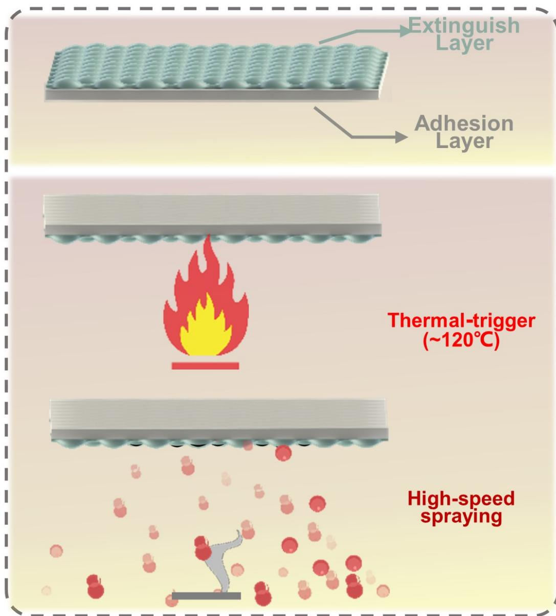
**Fig. S4** Composition of fire extinguishing patch and its fire extinguishing principle schematic diagram.
