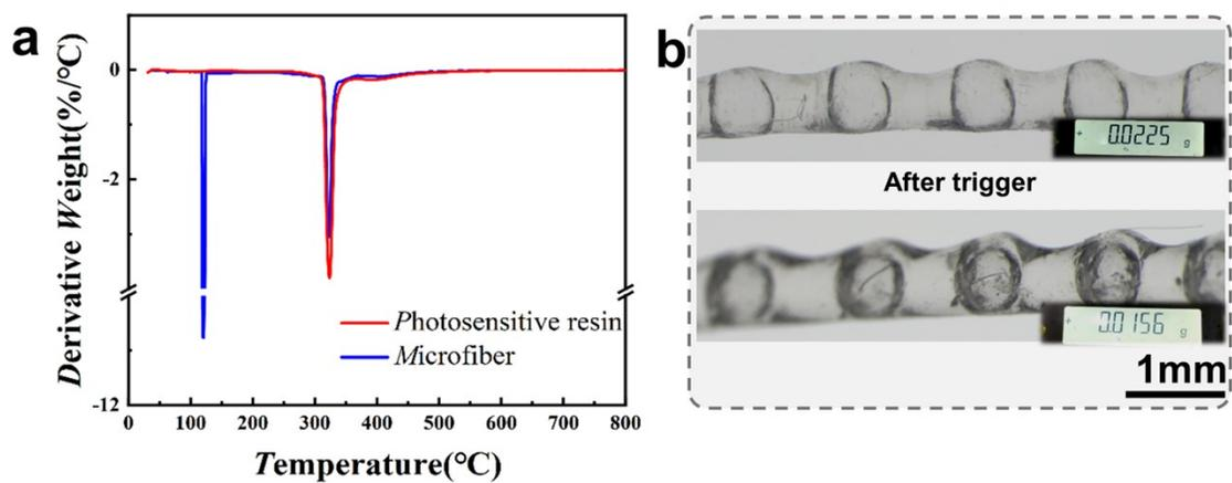
**Fig. S3** (a) DTG curve of photosensitive resin and FEMFs. (b) Mass change of a section of FEMF before and after release of extinguishing agent.
