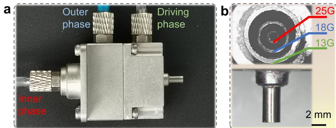
**Fig. S1** (a) Diagram of coaxial flow spinning equipment. (b) Detail of coaxial capillary tubes.
