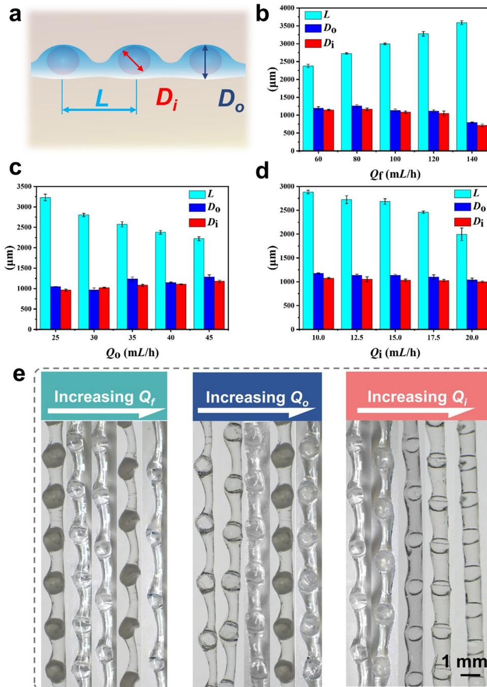
**Fig. S2** (a) Microfiber morphology parameters. (b) Effect of  $Q_f$  on microfiber morphology parameters ( $Q_i=10$  mL/h.  $Q_o=40$  mL/h). (c) Effect of  $Q_o$  on microfiber morphology parameters ( $Q_i=10$  mL/h.  $Q_f=40$  mL/h). (d) Effect of  $Q_i$  on microfiber morphology parameters ( $Q_o=10$  mL/h.  $Q_f=40$  mL/h). (e) Optical micrographs of the corresponding fibers in (b-d).
