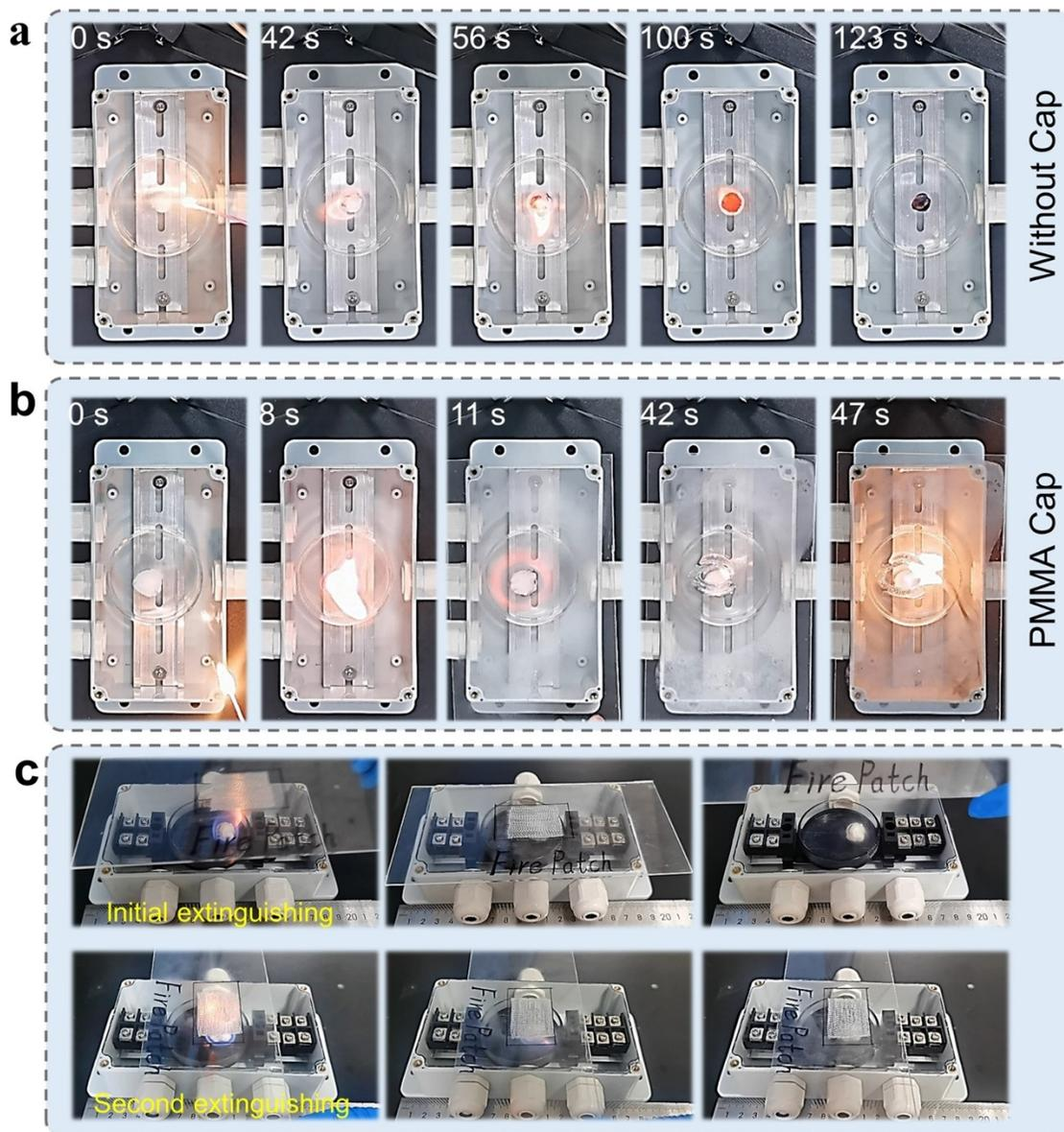
**Fig. S6** (a) The simulated fire source continues to burn for 120 seconds in an open environment. (b) The simulated fire source burns through the PMMA cover. (c) The FEP extinguishes the simulated fire source multiple times.
