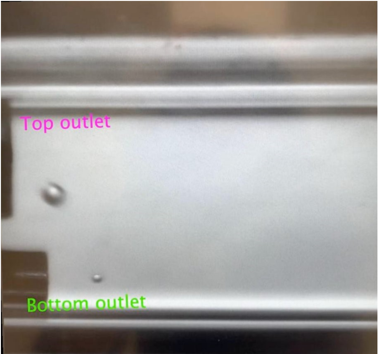
Video S1: Sorting of PS and PMMA mixture at 50 \mu\text{L}/\text{min} and 10 \mu\text{L}/\text{min} flow rates for top and bottom outlets, respectively, in a levitation media containing 0.01% of Pluronic and 75 mM Gd in PBS.
