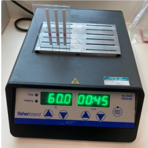
Figure S4. A picture of the developed device inserted in the heat block to run the optimised multiplex loop-mediated isothermal amplification (LAMP) assay for detection of Staphylococcus aureus enterotoxin A and B genes in raw ruminants' milk.
