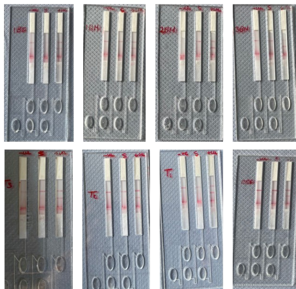
Figure S13. Field testing of (A) individual and (B) bulk tank milk samples for the detection of Staphylococcus aureus enterotoxins A and B genes using the developed microfluidic device. A
