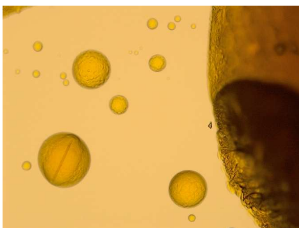
Figure S16. Partial crystalline behavior of the dipentoxo-AAP 2e under a light microscope with 10x magnification after irradiation with UV-light ( \lambda = 365 \text{ nm} , 2 min).
