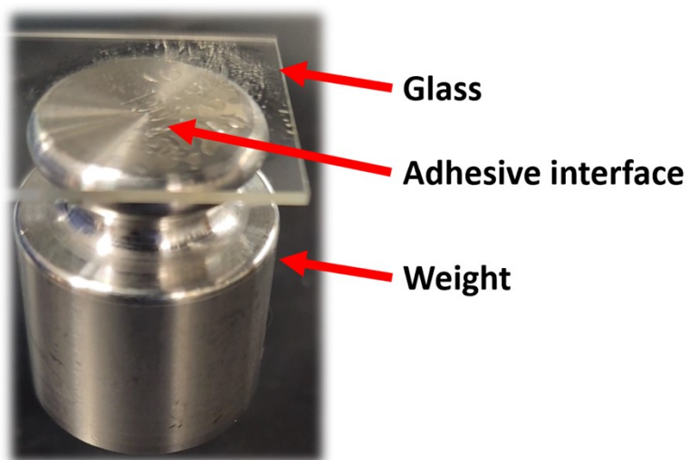
Figure S20. Photograph showing adhesively bonded glass and weight used for demonstrating the tackiness of the adhesive. The adhesive was prepared with p(HEMA-co-SHAM 10 ) and PVDF mixture with a copolymer to PVDF weight ratio of 85:15, an overlapped area of 258 mm 2 and a coating density of 4 mg/cm 2 .
