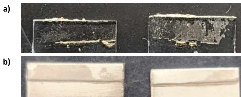
Figure S14. Image of (a) glass and (b) titanium substrates after performing the lap shear adhesion test tested with p(HEMA-co-SHAM 10 ). The adhesives were prepared by maintaining a copolymer to PVDF weight ratio of 85:15 with an area of joint overlap of 64.5 mm 2 and a coating density of 4 mg/cm 2 .
