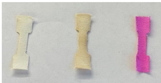
Figure S17. An optical image of untreated plain cotton (left), PEAA-8C-NH 2 solution-treated cotton with TPP removed (middle), and PEAA-8C-NH 2 solution-treated cotton after RB treatment (right).
