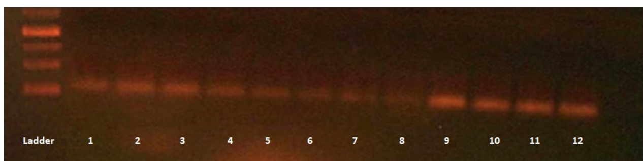
Fig. S13. Gel electrophoresis in 1% w/v agarose gel-to assess the efficient binding of GFP-mRNA onto the magnetic nanoparticles. Lane 1: NPs-Ch GFPmRNA (ratio: 1/0.5); Lane 2: NPs-Dx GFPmRNA (ratio: 1/0.5); Lane 3: NPs-Dx GFPmRNA (ratio: 1/3); Lane 4: NPs-Ch GFPmRNA (ratio: 1/3); Lane 5: NPs-CA-Ch GFPmRNA (ratio: 1/0.5); Lane 6: NPs-CA-Ch GFPmRNA (ratio: 1/1.5); Lane 7: NPs-CA-Ch GFPmRNA (ratio: 1/3); Lane 8: NPs-CA-Ch GFPmRNA (ratio: 1/5); Lane 9: NPs-CA-Dx GFPmRNA (ratio: 1/0.5); Lane 10: NPs-CA-Dx GFPmRNA (ratio: 1/1.5); Lane 11: NPs-CA-Dx GFPmRNA (ratio: 1/3); Lane 12: NPs-CA-Dx GFPmRNA (ratio: 1/5).
