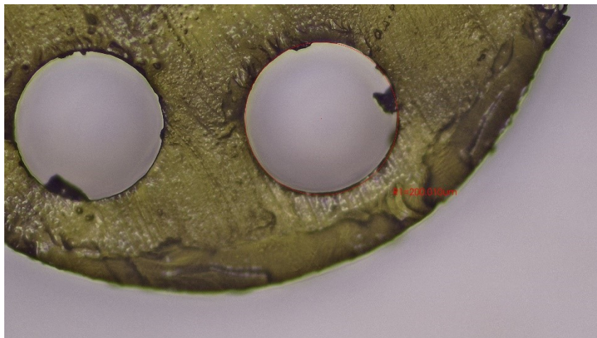
Fig. S4. Inner diameter of the 7-channel NGC measured under optical microscopy( R=200.010\mu\text{m} )
