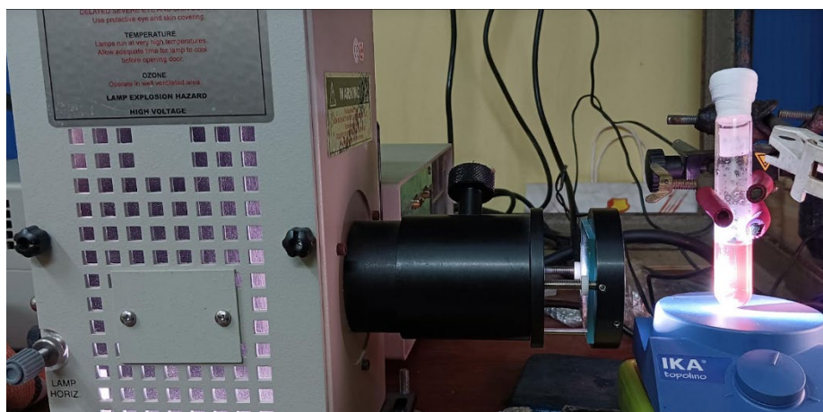
Fig. S16: Experimental set up of photocatalytic H 2 evolution.
