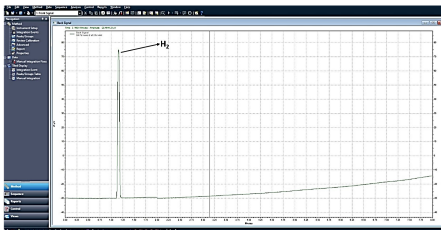
Fig. S15: Gas chromatograms: The peak of hydrogen evolution for CTF-TPP@Pd 0.5 applying 2 mg photocatalyst, 5 mL water, 1 mL TEOA and 4 mg EY.
