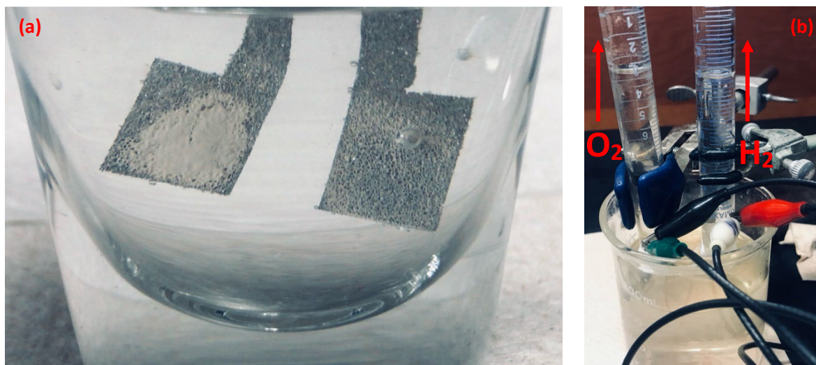
Figure S14: Digital Photograph of (a) the two-electrode symmetric cell electrolyzer, and (b) digital image of the setups for O 2 and H 2 gas collection using a measuring cylinder.
