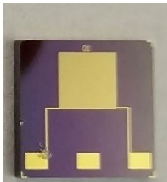
Figure S 2. An image for the IDE electrode used for the material deposition.
