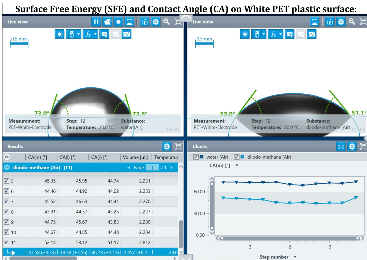
(A) Contact Angle of test liquids on White PET plastic surface.
