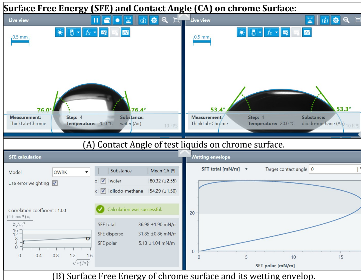
Figure S-3. Contact Angle and Surface Free Energy measured on chrome Surface using the KRÜSS MSA (Mobile Surface Analyzer). (A) Contact Angle of test liquids, water and diiodo-methane on chrome surface. (B) Surface Free Energy calculation (SFE total, SFE disperse and SFE polar) using Owens, Wendt, Rabel and Kaelble (OWRK) method along with wetting envelop plot.
