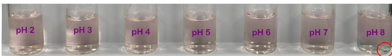
Figure S4 A solubility test for \text{Co}^{2+} in aqueous solutions at 25^\circ\text{C} with varying pH values.
