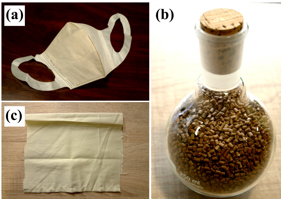
Figure S2. Digital images of (a) a facemask made of Cu 2 O NP-PP meltblown nonwoven fabrics using Cu 2 O NP-embedded PP masterbatches as raw material. (b) Cu 2 O NP-embedded PET masterbatches that can be used to fabricate Cu 2 O NP-PET meltblown nonwoven fabrics as demonstrated in (c).
