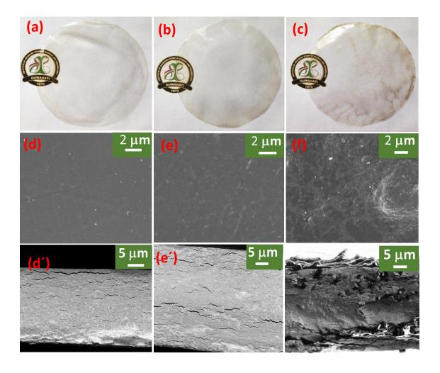
Figure S1. (a), (b), and (c) are the photograph of 0.12% CNF-SA, 1% CNF-SA, 4% CNF-SA film; (d-d'), (e-e'), and (f-f') are the SEM image of 0.12% CNF-SA, 1% CNF-SA, 4% CNF-SA film.
