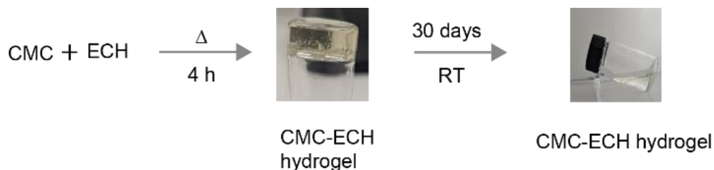
Figure S4. Gelation of CMC and epichlorohydrin (ECH) at 70 °C for ~4h. Photographs of reaction mixture and vial inversion test giving stable gel matrix. Dissolution of hydrogel was observed after 30 days at room temperature.
