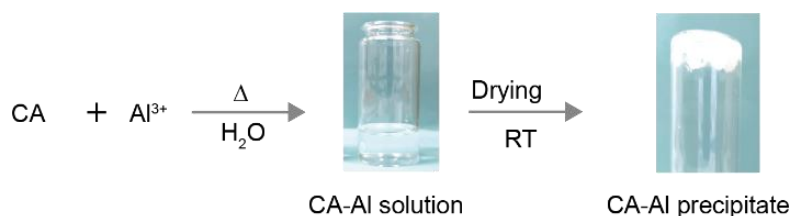
Figure S10. Schematic of a reaction between CA powder and \text{Al}^{3+} ions in water with photographs showing clear solution which formed a precipitate upon drying.
