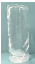
Figure S2. CMC 2wt% (or above) in water, leading to a highly viscous, but poor gelation.
