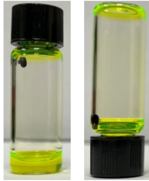
Fig. S9. 500 \mu M QGTsfGFP after being frozen at -80 ^{\circ} C and thawed at 4 ^{\circ} C. Vial inversion demonstrated that QGTsfGFP under these conditions flowed due to gravity and did not form a gel.
