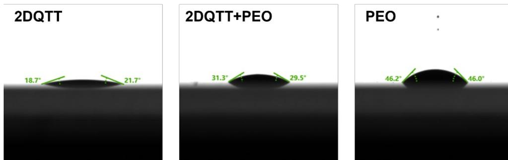
**Figure S2** The contact angle changes of 2DQTT, PEO and their mixed solution droplets on the glass substrate surface.
