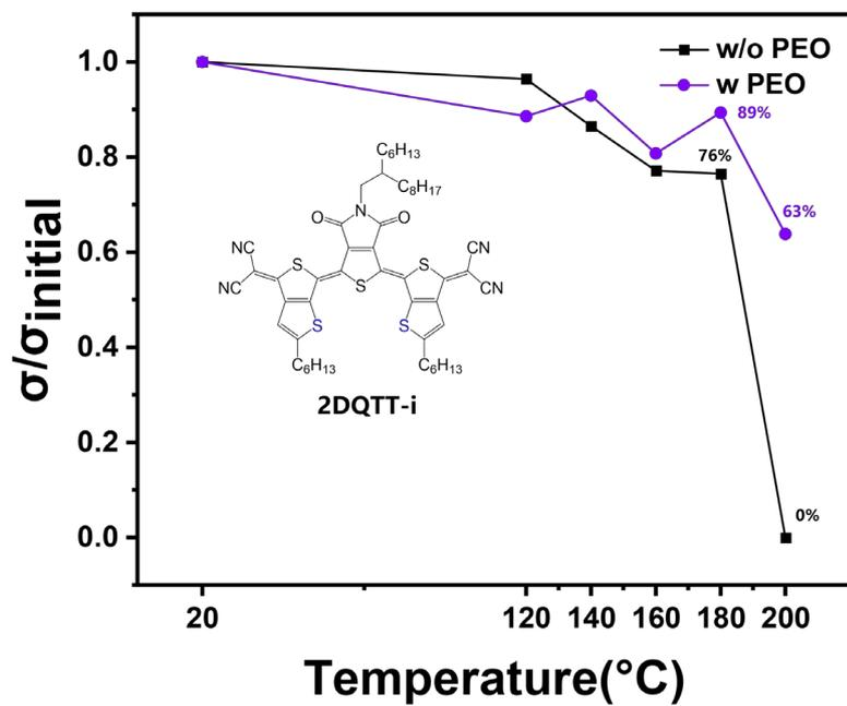
**Figure S8** Attenuation ratio of electrical conductivities of doped 2DQTT-i after heating at different temperatures.
