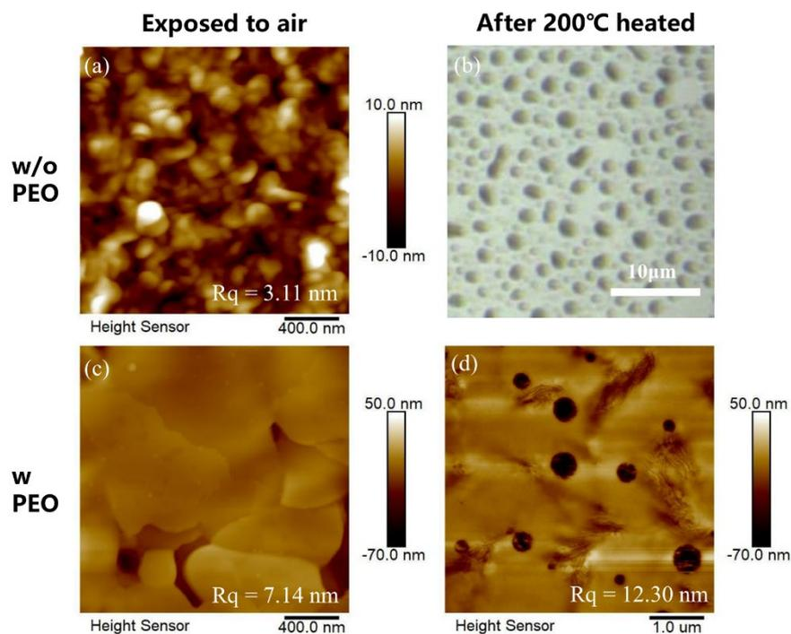
**Figure S6** Atomic force microscopy (AFM) images of the 2DQTT-o films doped by N-DMBI a) without PEO exposed to air and c) with PEO exposed to air; d) doped by N-DMBI with PEO after heating at 200 °C. b) Optical microscope image of 2DQTT-o doped film without PEO after heating at 200 °C (The AFM image is unable to obtained due to the large roughness).
