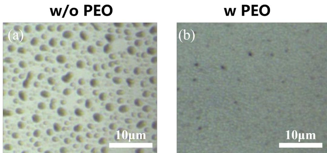
**Figure S7** Optical micrograph of 2DQTT-o doped film after heating at 200 °C : a) without PEO and b) with PEO.
