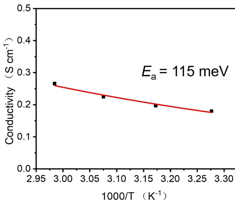
**Figure S3** The electrical conductivity of 2DQTT-o doped films with PEO changed with temperature.
