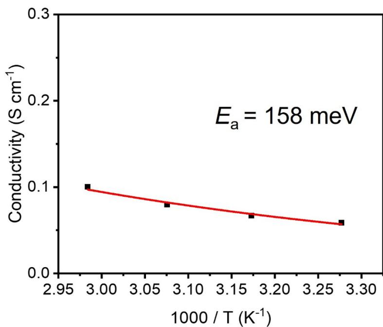
**Figure S4** The electrical conductivity of 2DQTT-o doped films without PEO changed with temperature.
