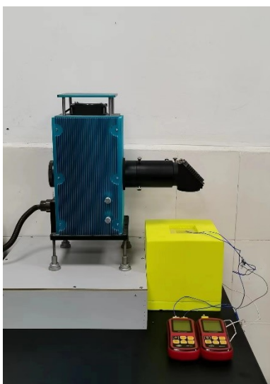
Figure S8 Photograph of model house in using PBA ion gels as smart windows.
