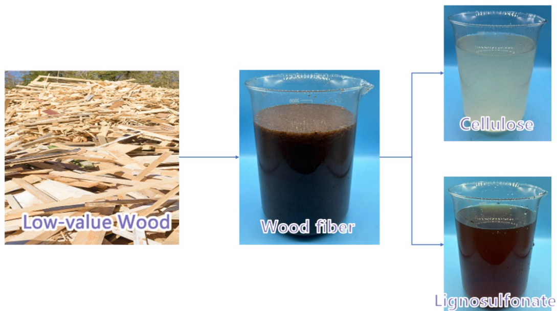
Fig. S3. The wood processing residue is put into a colloidal mill to grind into a fibrous pulp. The wood fiber is treated with sodium hydroxide and sodium sulfite, and the waste liquid after filtration is treated to get sodium lignosulfonate. The treated wood fibers are bleached and pulped to obtain cellulose.
