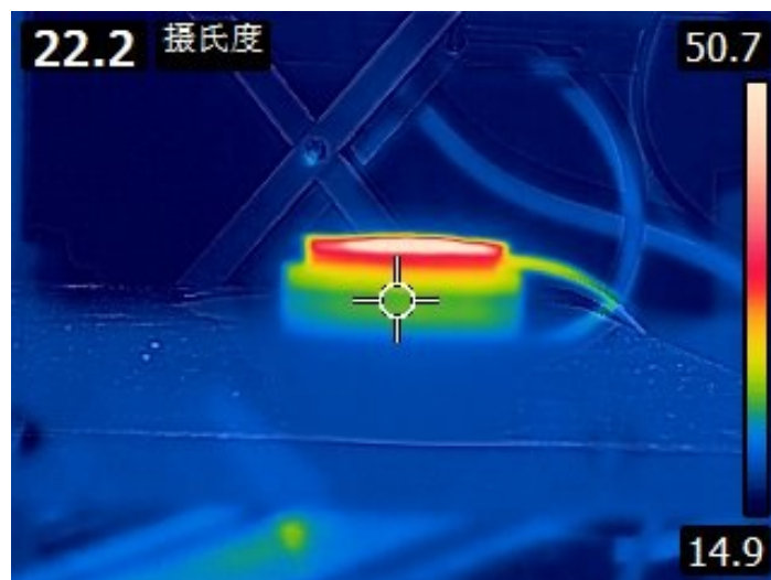
Fig. S15. Infrared images of the TEG under 0.1 \text{ W cm}^{-2} illumination.
