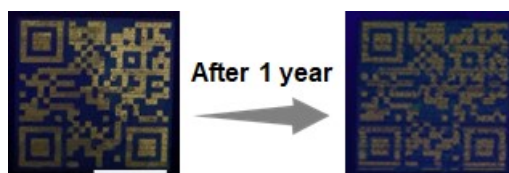
Figure S24. Fluorescent images of the printed QR code before and after storage for one year (Scale bar: 1 cm).
