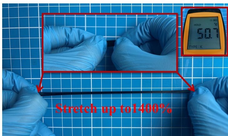
Fig. S9 The photographs demonstrate that the ASSICEs exhibit a tensile strength of up to 1400% at a temperature of 50 °C.
