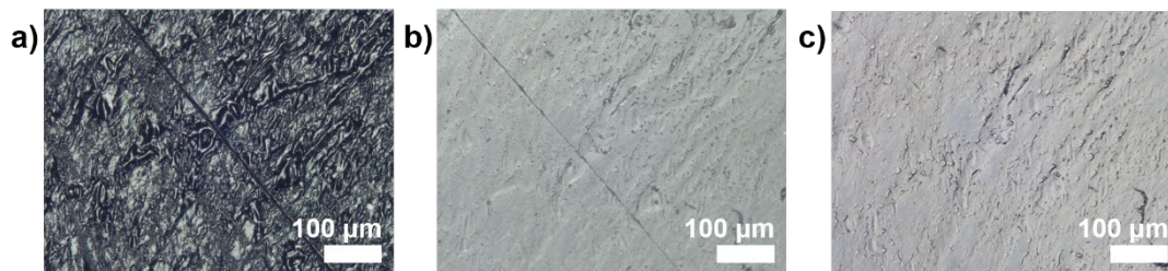
Fig. S19. Visual inspection of the self-healing behavior of PEDOT/RILNs-2. (a) Scratched sample, (b) healed sample (healing conditions: 150 °C, 60 min), and (c) healed sample (healing conditions: 150 °C, 90 min).
