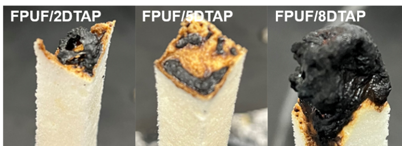
Fig. S6. Digital photos of LOI test for FPUF/2DTAP, FPUF/5DTAP and FPUF/8DTAP.
