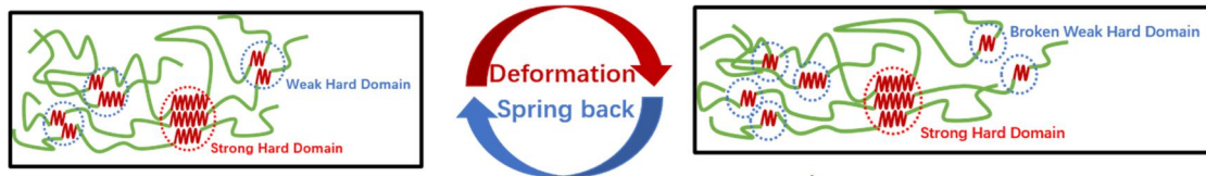
Figure S29. Illustration of rebound caused by coiling of the soft segments and reconstruction of the hard domains.
