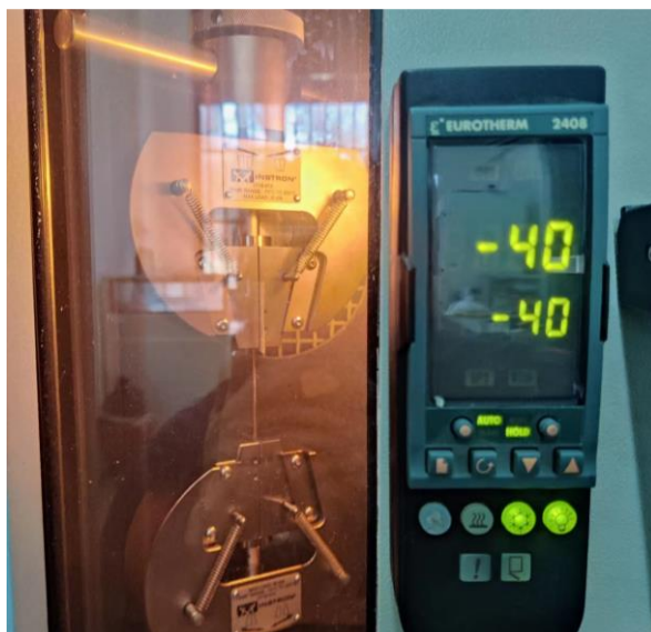
Figure S23. Photograph of P-GHK stretched at -40\text{ }^{\circ}\text{C} .
