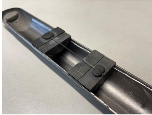
Figure S10. Setup and attaching of fiber rovings with a length of 5-8 cm with mullite glue on carbon pieces inside quartz glass crucibles. Left: oxidize PAN/OSZ-40 fibers before pyrolysis; right: pyrolyzed C/SiCON-40 fibers.
