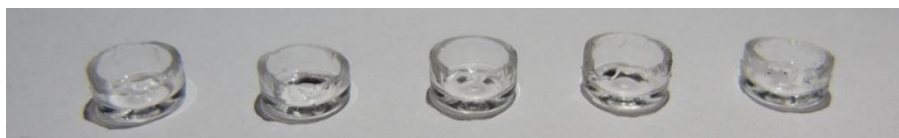
Figure S7. Cut glass vials for the measurement of the transmittance of the glass bottom. Adapted from a previous publication. 3-5
