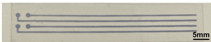
1 2 Figure S35. Digital image of the 2-channel electrode prepared by combining the stencil-printing 3 and the proposed method.
