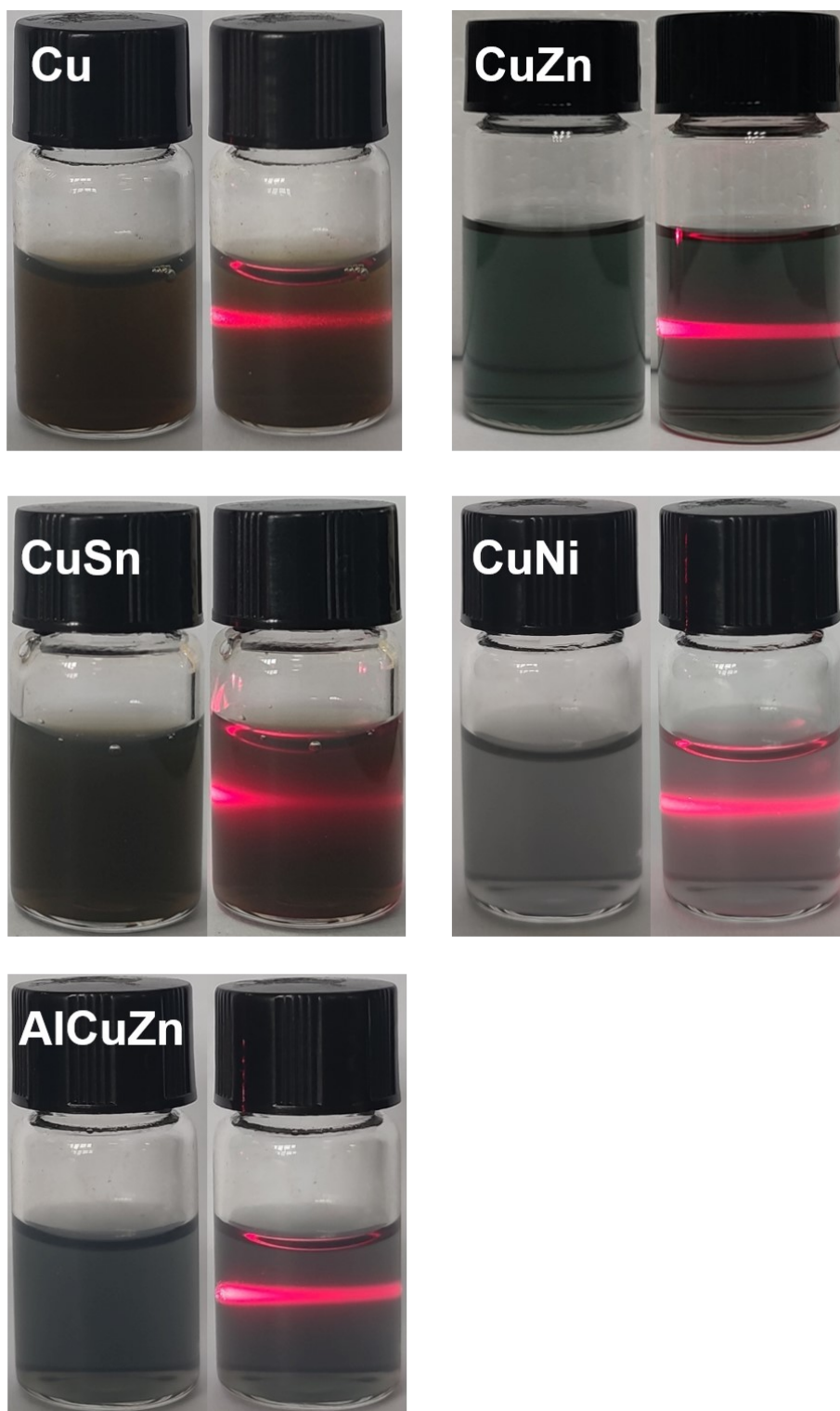
Fig. S3 Dispersion images of copper-based metallenes. Photographs of copper-based metallene dispersions with /without laser.
