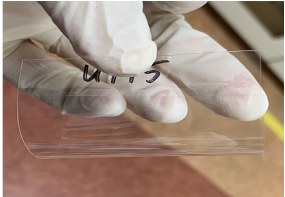
2 Fig S5. Coating tests of AUP@SiOx-184 and AUP@SiOx solutions on glass and PET 3 substrates, respectively.
